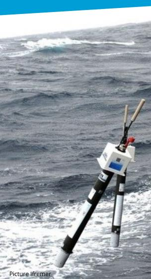
**ARVOR I** provides salinity, temperature and pressure profiles with position information thanks to an integrated GPS receiver. Data are transmitted via Iridium satellites network.
