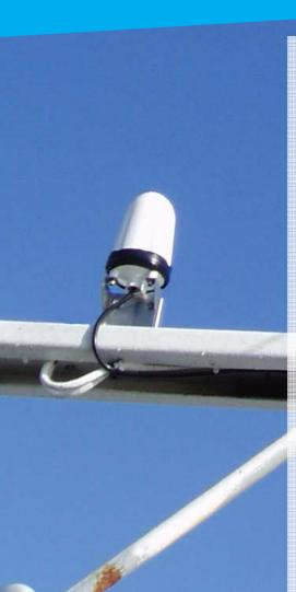
Installed aboard the ship, **NAVLOC** beacon can automatically receive and send the boat position at regular rates. Out of the maintenance of the NAVLOC beacon, no operation is required for the crew to operate.
