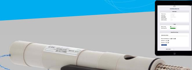
**WiSens CTD** measures and records **conductivity**, **temperature and depth.** Salinity is deducted by calculation. It has been designed to be used down to 300m.
