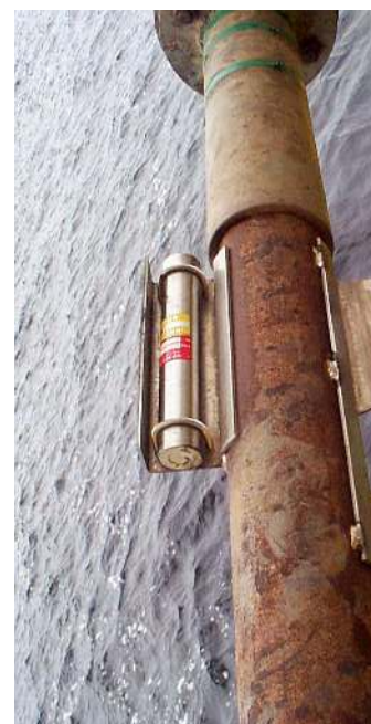
Mounting of WiSens-DA on a corer
