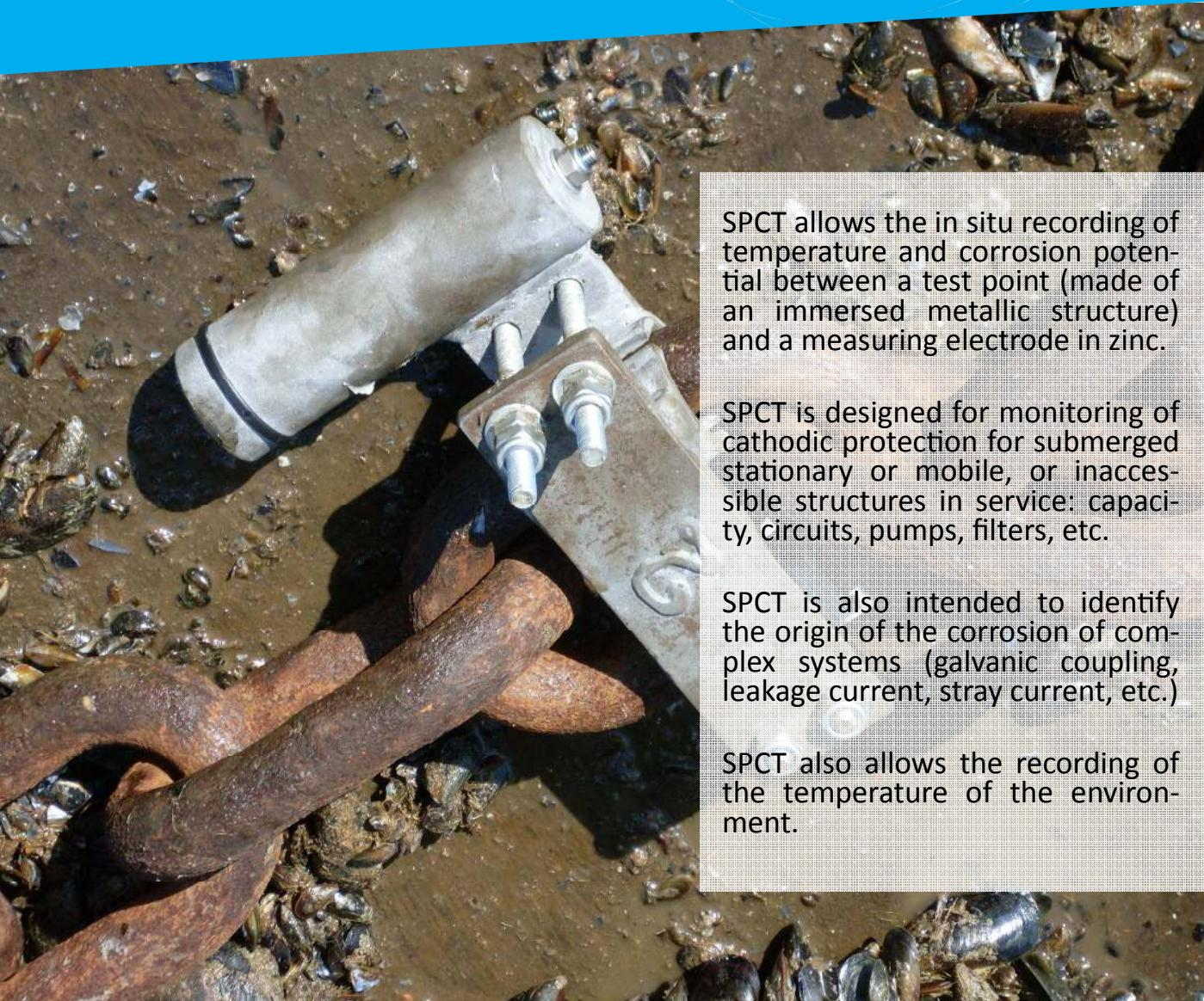
SPCT allows the in situ recording of temperature and corrosion potential between a test point (made of an immersed metallic structure) and a measuring electrode in zinc.
