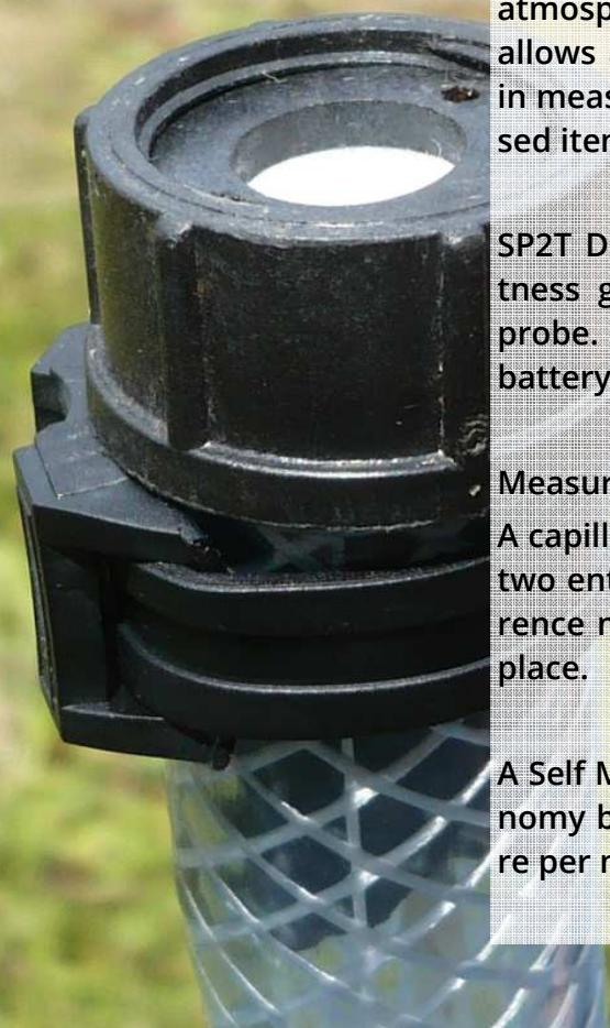
This logger enables to measure a difference of height between any two points. In tide gauge function, the measure is realised between the sea bottom and the atmosphere. A correction of the atmospheric pressure allows a higher accuracy. Another application consists in measuring the vertical distance between two immersed items.
