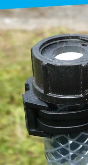
This logger enables to measure a difference of height between any two points. In tide gauge function, the measure is realised between the sea bottom and the atmosphere. A correction of the atmospheric pressure allows a higher accuracy. Another application consists in measuring the vertical distance between two immersed items.
