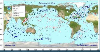
These drifters are used mostly offshore in order to monithe current ať sea surface tor for tor the current at sea surface for oceanographic studies and also the oil spill trajectories. The drifters can be fitted with holey socks drogue and are, by this way, linked to a particular mass of water. The drag ratio between surface buoy and the drogue validates the good function of current follower. If no drogue is mounted, the drifter is affected by the sur-face current face current.
